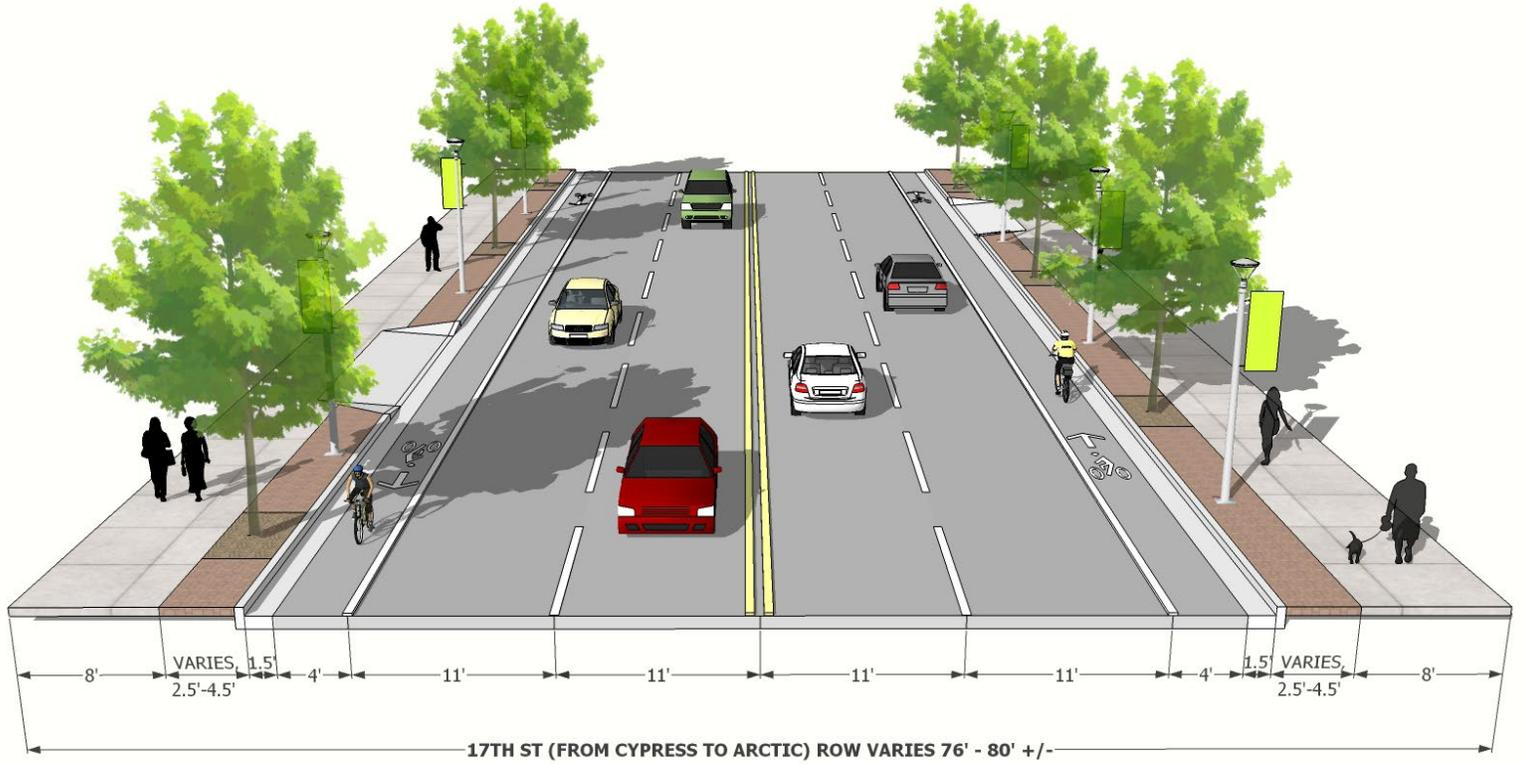
FIGURE 7. 17TH STREET PROPOSED SECTION B - ON STREET PARKING
