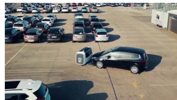
FIG. 4.1.11 AUTOMATED, SELF-VALET © Stanley Robotics
