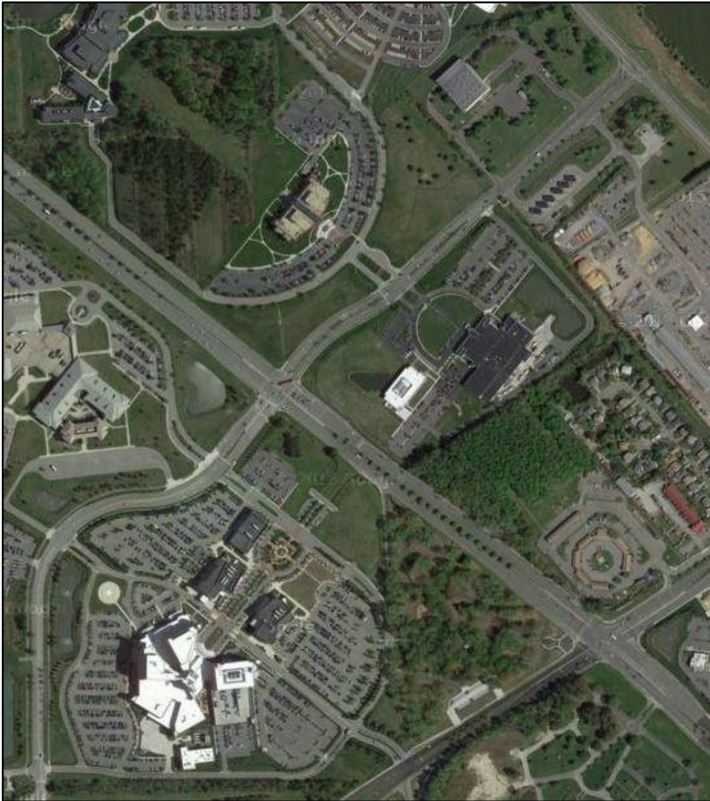
Area with several projects that demonstrate the use of good internal access to parking lots with limited access points to arterial roadways
