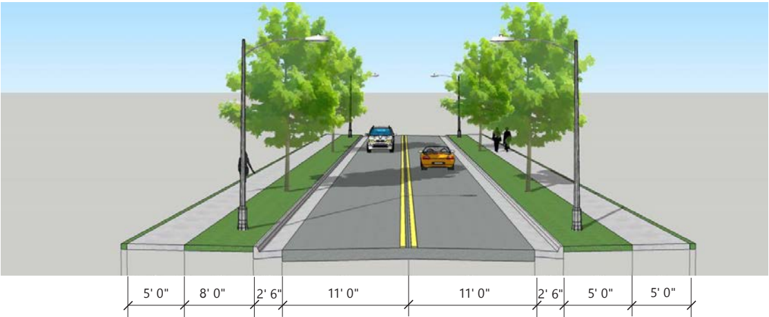
BURTON STATION ROAD TYPICAL SECTION
